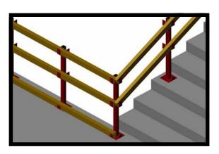
This post can be used in a variety of situations on a building site as a Temporary safety barrier or hand railing across landings and stairs.
